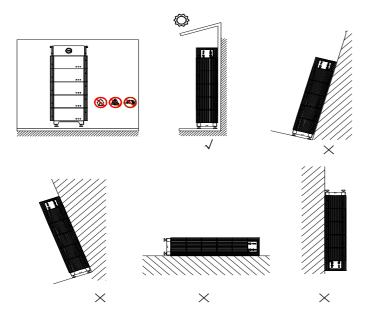
Figure 4.3 Mounting method
