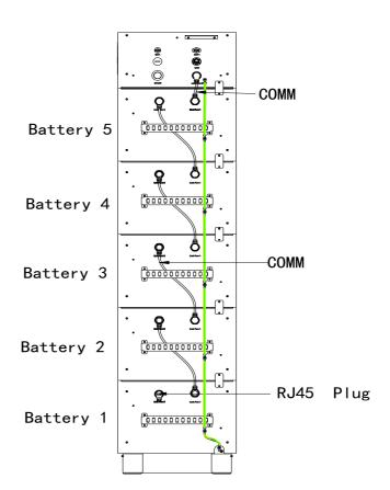
Figure 5.3 Connecting battery COMM cable
