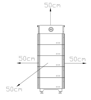
Figure 4.1 Installation location
