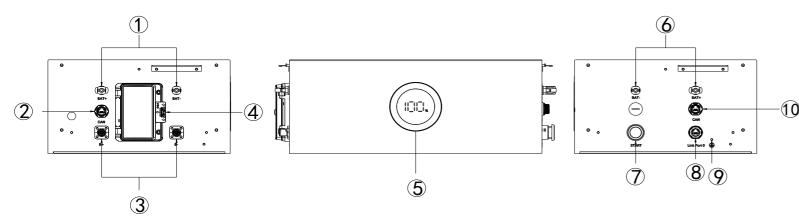
Figure 3.3 Battery control unit interface (left view and right view)
