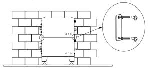
Figure 4.6 Securing battery modules with locking brackets
