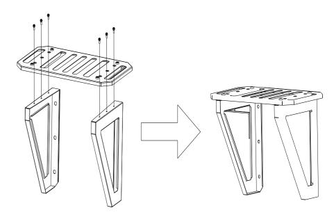
Figure 4.9 Assembling the bracket
