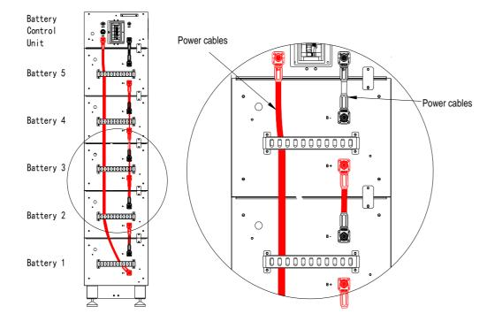
Figure 5.4 Connecting battery power cables
