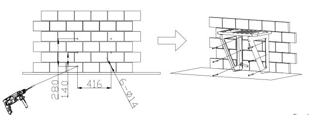
Figure 4.11 Install the locking bracket
