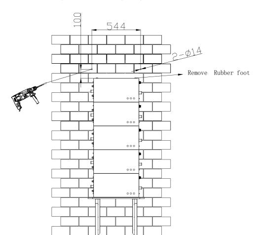
Figure 4.13 Installing battery control unit
