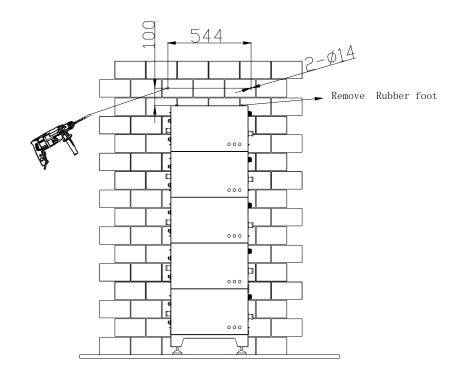
Step 3: Stack the rest of the battery modules up and secure the battery modules with locking brackets
