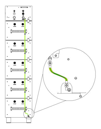
Figure 5.2 Connecting the additional grounding cable
